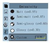
As shown in the figure, press " MENU " key to enter the main menu and select "  $\, \xi \,$  " (emissivity) option and press "  $\, \blacktriangleright \,$  " key to enter the emissivity list.
