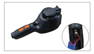
Take care to slide the battery cover into the correct position of the handle.
